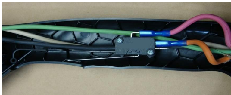
Fig. 6-5 Switch Wire Location
